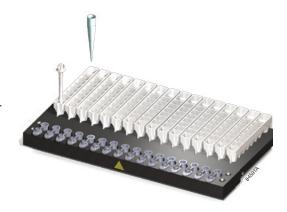
**Figure 1.** The LEV Plunger is placed in Well #8 of the cartridge (the well closest to the Elution Tube), and lysates are placed into Well #1 of the cartridge.
