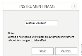
Figure 133. 'Instrument Name' screen. Administrators can manually enter the instrument name from the 'Instrument Name' screen.
