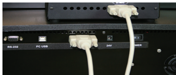
Figure 119. Cable connection of injector system to GloMax® Discover Instrument.
