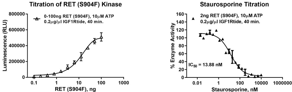
**Figure 3. RET (S904F) Kinase Assay Development.** (A) RET (S904F) enzyme was titrated using 10 $\mu$ M ATP and the luminescence signal generated from each of the amounts of the enzyme is shown. (B) Inhibitor dose response was created using 2ng of RET (S904F) to determine the potency of the inhibitor ( $IC_{50}$ ).
