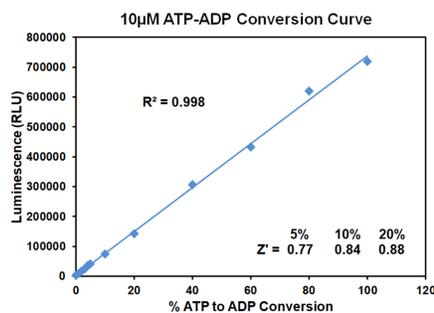
**Figure 2. Linearity of the ADP-Glo Kinase Assay.** ATP-to-ADP conversion curve was prepared at 10µM ATP+ADP concentration range. This standard curve is used to calculate the amount of ADP formed in the kinase reaction. Z' factors were determined using 200 replicates of each of the % conversions shown.
