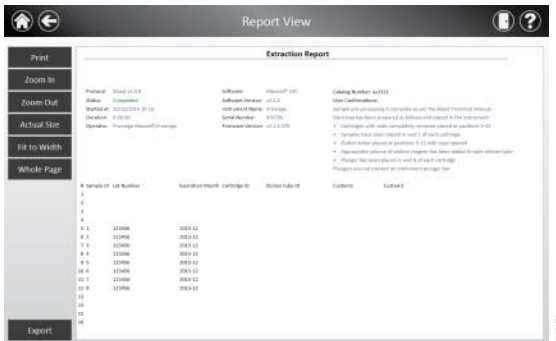
Figure 58. Extraction Report. An example of the sample tracking information present in an extraction report as well as Exporting reports.
