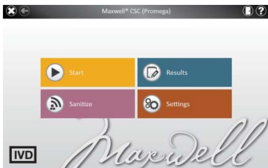
Figure 36. Maxwell® CSC Home screen. Selecting the Start button begins the process of running a protocol on the Maxwell® CSC Instrument.
