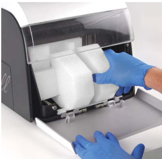
Figure 7. Remove the two foam pieces from inside the instrument.
