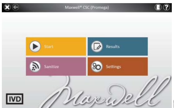
Figure 56. Maxwell® CSC Home screen. Selecting Results opens the Maxwell® CSC ‘Reports’ screen from which extraction reports from all extraction runs, service activities, and system activities can be viewed.
