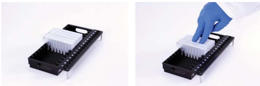
Figure 43. Place the cartridges in the deck tray, and press firmly to snap them in place.
