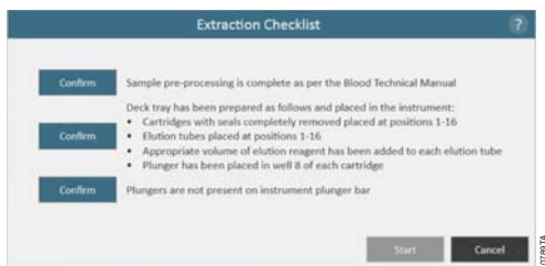
Figure 42. Extraction Checklist screen. This screen indicates the steps that will need to be performed to prepare the instrument for processing the selected samples. Preprocessing steps are not indicated on the 'Extraction Checklist' and should be performed prior to this stage according to the technical manual for the kit being processed.
