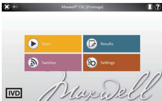
Figure 22. Maxwell ® CSC Home screen. Selecting Settings opens the Maxwell ® CSC 'Settings' screen from which bar code entry options can be configured.
