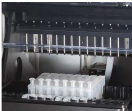
Figure 4. Magnetic assembly components and platform. The hardware components inside the Maxwell® CSC Instrument. The magnet and plunger bars, which are used for sample processing, and the platform containing the deck tray are evident.
