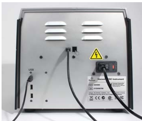
Figure 3. Rear view of the Maxwell® CSC Instrument. The rear of the instrument showing the On/Off switch, power cable connector, instrument-to-tablet USB communication port and three additional USB communication ports for peripherals (e.g., Bar Code Reader).
