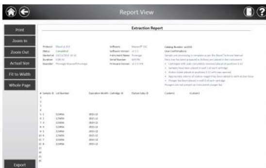
Figure 52. Report View screen. The 'Report View' screen displays the sample tracking and protocol-specific information for the current instrument run. Included in this report are the sample tracking information recorded prior to starting the protocol, the final status of the protocol (Completed or Aborted), the time the protocol run was started, the length of time the protocol took to process, the operator ID and additional instrument information. In the lower left corner of the screen is an Export button that will be used for exporting report information.
