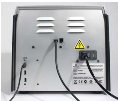
Figure 12. Connect the Tablet PC to the back of the Maxwell ® CSC Instrument.
