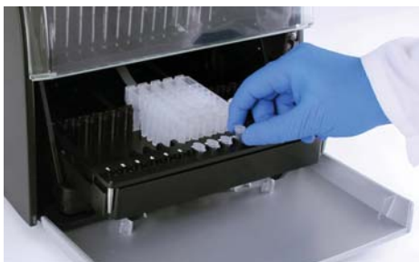
Figure 49. Removing the elution tubes and the deck tray.
