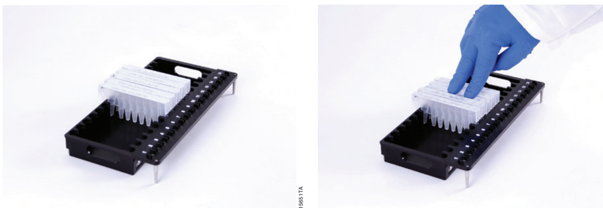
Figure 29. Placing the cartridges in the Deck Tray and pressing firmly to snap in place.
