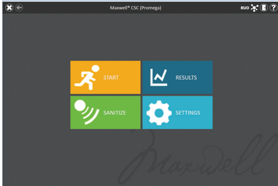
Figure 43. 'Home' screen. Selecting the Sanitize button begins the process for UV treatment of the Maxwell® CSC Instrument.
