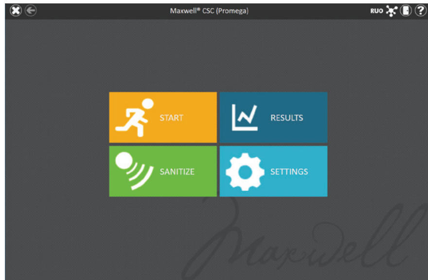
Figure 40. 'Home' screen. Selecting Results opens the 'Results' screen from which extraction reports from all method runs can be viewed.
